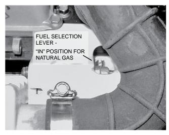
Figure 2. 10 kW, GT-530 (Inlet Hose Slid Back)
